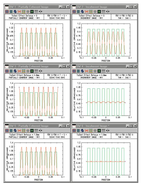
We can also examine the incoherent in-focus image of the square wave using the modulation transfer function. The image modulation of a square wave of frequency  $f_0$  can be computed by resolving the square wave into its Fourier (i.e., sine wave) components and using the MTF value for each sine wave frequency. The resulting square wave modulation  $S(f_0)$  is given by
